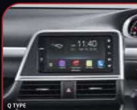
TOUCH SCREEN AUDIO SYSTEM 7" DVD AVX w/ MP3/USB/AUX/iPod with Mirroring over Wi-Fi, Internet Browser, Voice Command (Q, V, & G TYPES)
